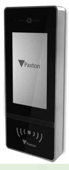
The Entry panel is a robust door entry panel incorporating both door entry and access control functions. It is powered using power over Ethernet (PoE) and communicates with the other elements of the system using IPv6, providing 'plug and play' installation. Each panel is associated with a Entry control unit which is the interface to the door hardware.
