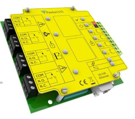
The Net2 I/O board is simple, yet powerful addition to the Net2 system. It can be wired alongside a Net2 door controller, to switch power on and off to electrical equipment to save money and energy. The board can control lighting, heating, water and air conditionoing by using the triggers and actions application in the Net2 software. These actions can be programmed for a particular time, or in response to a specific Net2 event.
