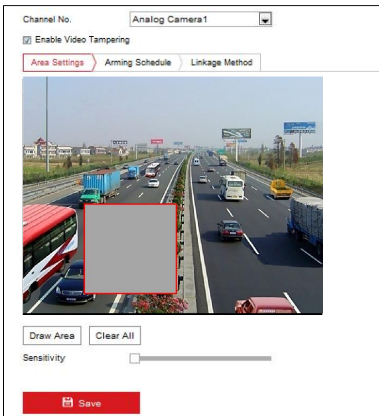
Figure 7. 15 Video Tampering Alarm Settings
