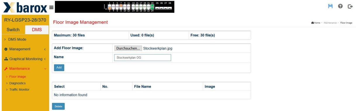
The uploaded plans are then listed in the lower section of the web page. Up to 50 files can be saved.
